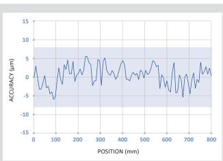
Accuracy graph: deviation between the value measured by the sensor and the value measured by the reference system.
