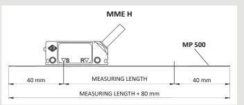
IMPORTANT: To guarantee the system accuracy, the magnetic band has to be 80 mm longer than the measuring length of the machine (40 mm for each side). During mounting, the magnetic band has to be adequately centered on the measuring length.
