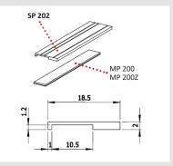
To be fixed on the machine to protect the magnetic band.
