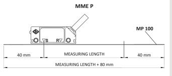
IMPORTANT: To guarantee the system accuracy, the magnetic band has to be 80 mm longer than the measuring length of the machine (40 mm for each side). During mounting, the magnetic band has to be adequately centered on the measuring length.
