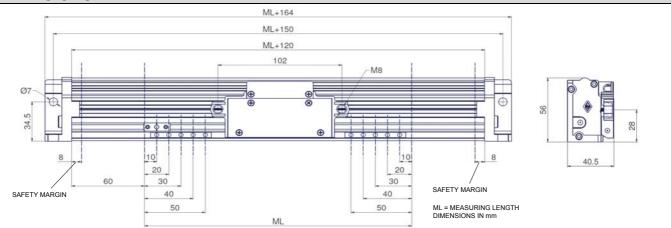
GV-PB adapter provided for the interchangeability with scale mod. PBS-HR.
